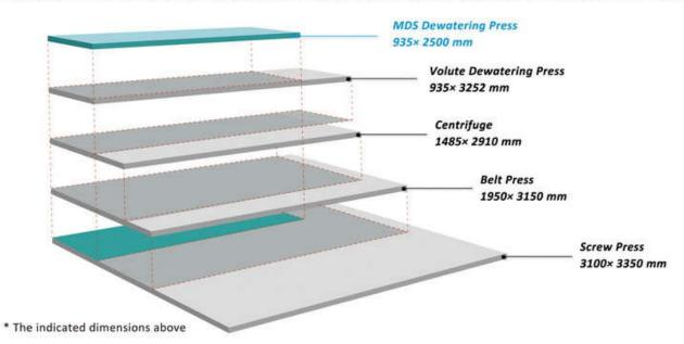
The shown dimensions for the belt press and centrifuge are for the main bodies only. For other dewatering equipment, the dimensions of attachments, such as PLC control panels, flocculation tank, etc. are also included.
